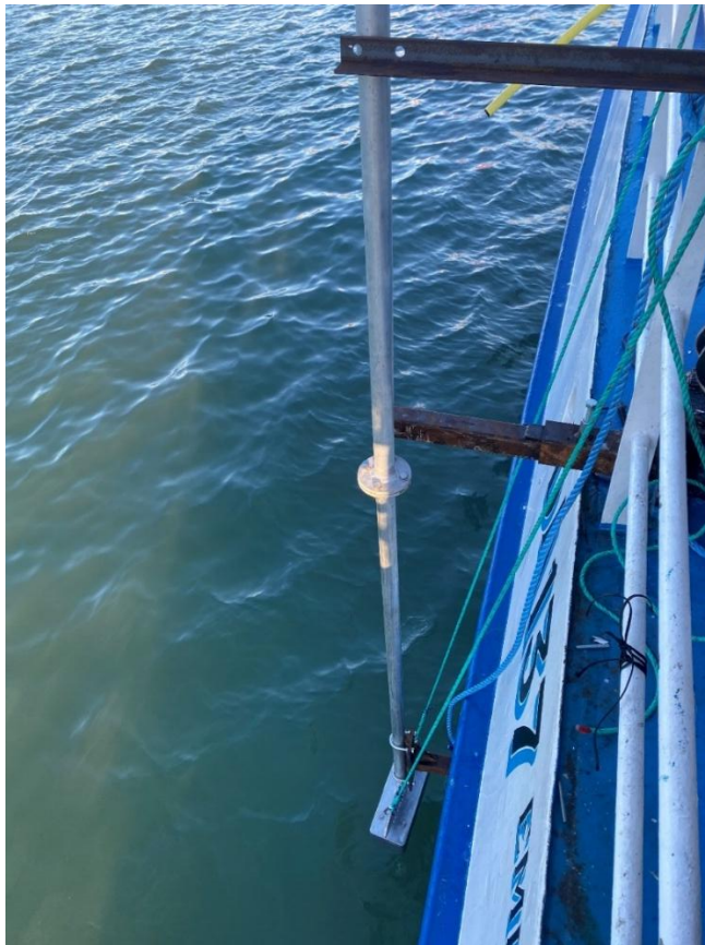
Figure 3. Over the side transducer pole mount (in raised position)
