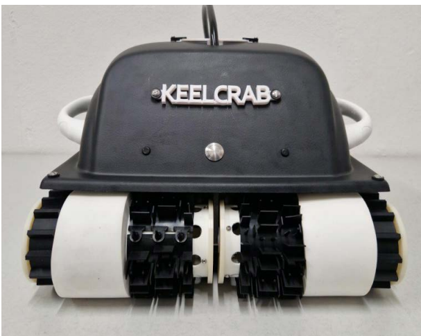
(Photo credit: Keelcrab.com; Hull drone cleaning device)
