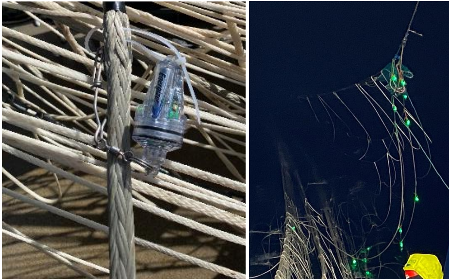
Figure 3. One of the green lights (Lindgren-Pitman) attached to the headline (left) and being deployed at night (right)
