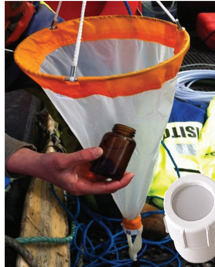
Figure 2. Phytoplankton net with sampling bottle and (inset) filter removed from base of net.
