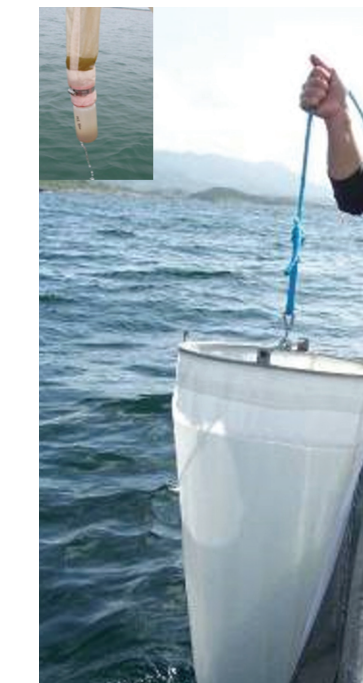
Figure 5. Zooplankton net being lowered into the water to collect sample. Inset top left: cod end of net with sampling bottle attached.
