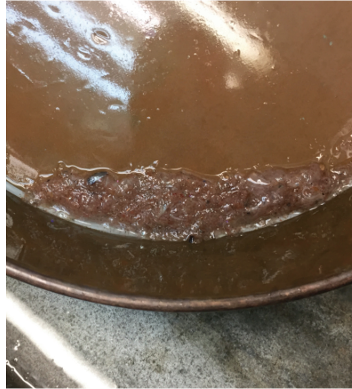
Figure 7. Sieve with 200- \mu\text{m} mesh used to filter sample and enable collection of zooplankton.
