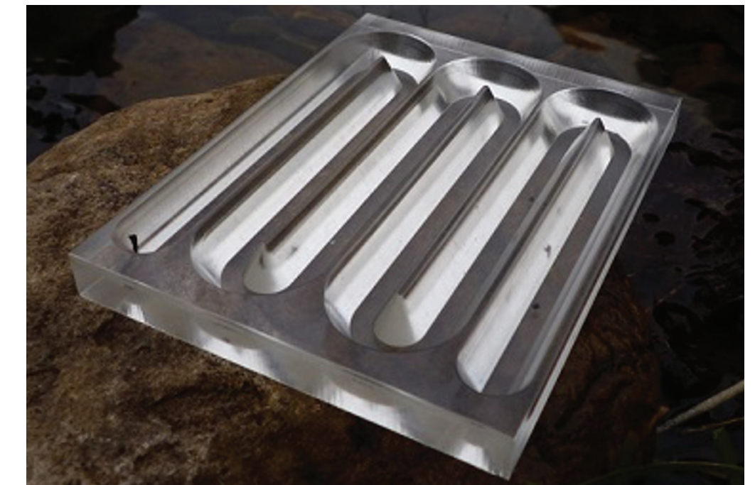
Figure 6. Bogorov tray used for counting zooplankton samples.
