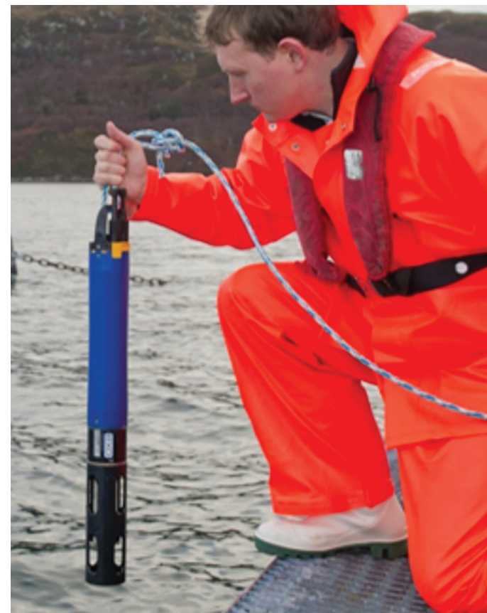
Figure 3. A Van Dorn sampler being lowered into the water.
