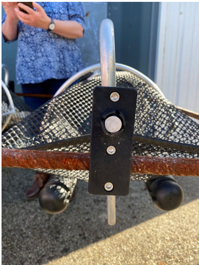
Figure 4: Fixed rotation bearing attached to trestle
