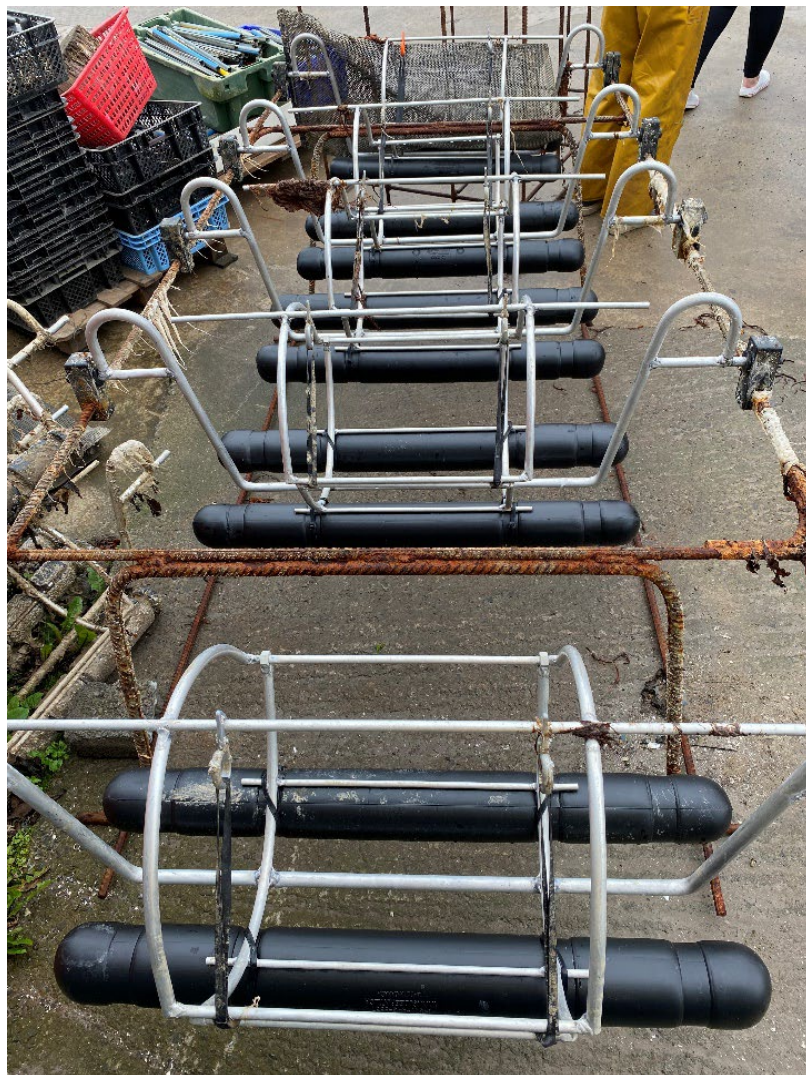
Figure 2: A single trestle with 5 turners fitted. Note the anti-sink bar on the trestle
