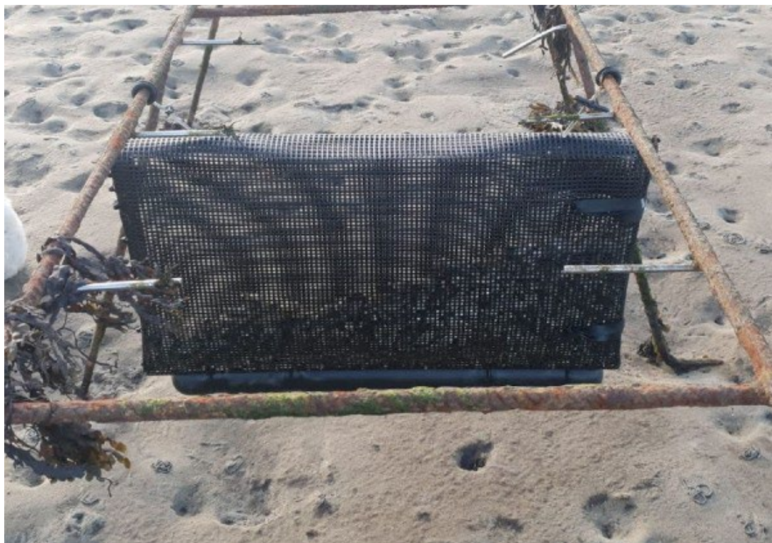
Figure 4: Modified trestle with short stainless steel bars welded horizontally to restrict the bag rotation to 180°
