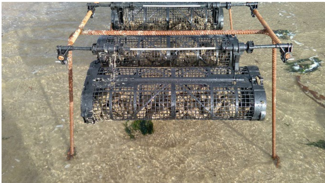
Figure 4: Seapa Basket clipped onto modified trestle www.seapa.com.au
