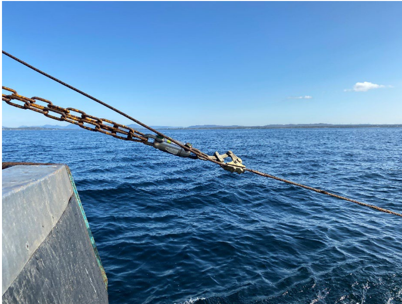
Figure 4. Loadcell with chain and gripper attached to warp.
