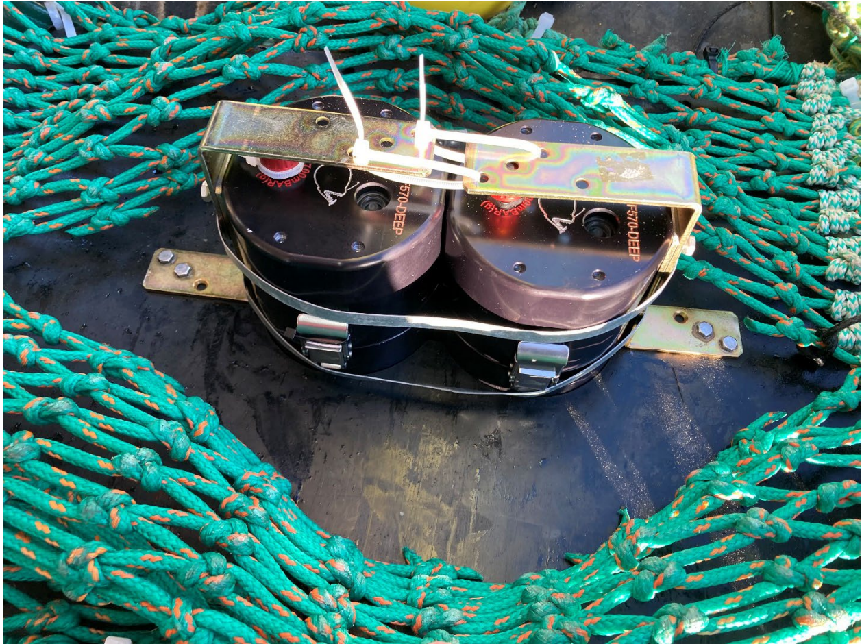
Figure 4. Nephrops trawl fitted with the Image Acquisition System (IAS) comprising: 4-panel tarpaulin; nylon mounting board; twin GoPro cameras in underwater housings; and SN Tech Pisces underwater lights.
