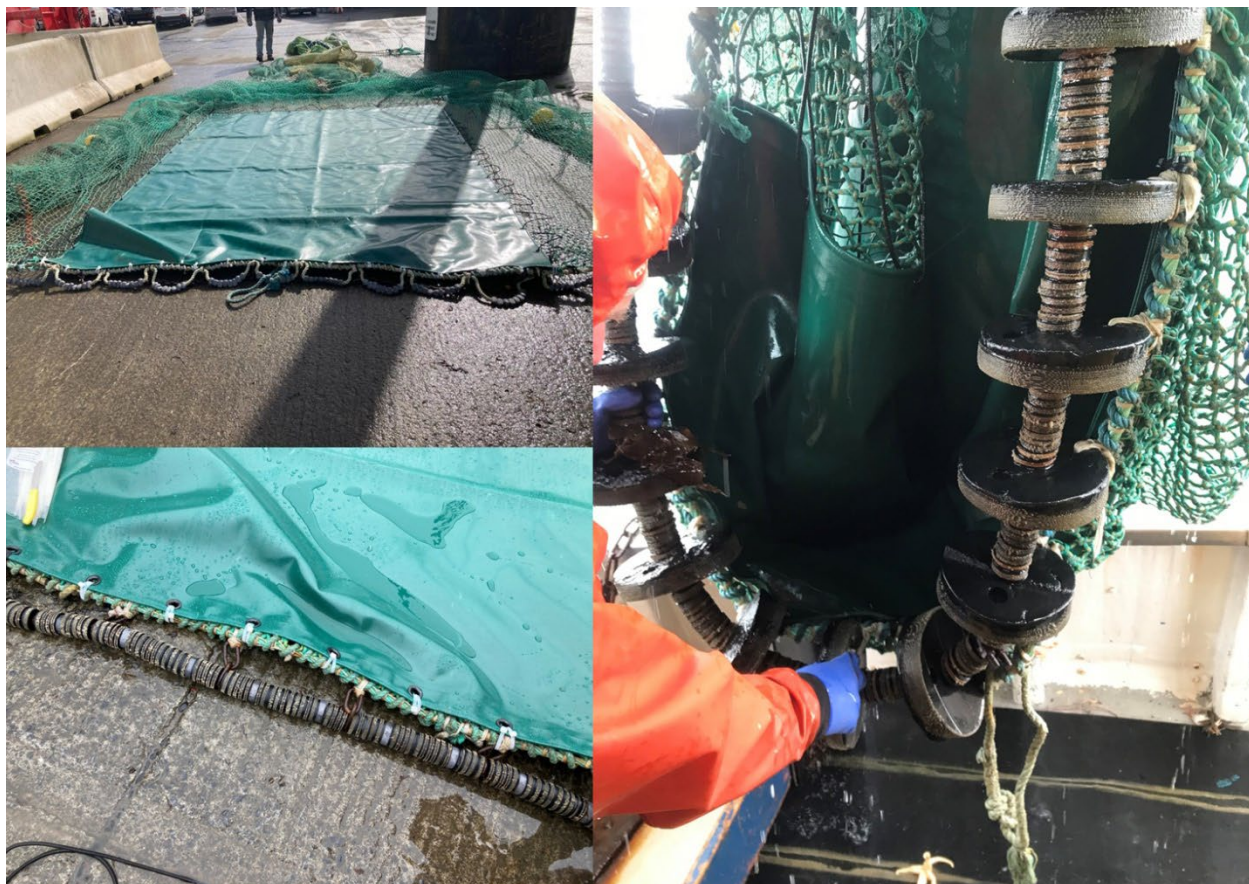
Figure 3. ground gear types deployed during trial (counterclockwise from top left): looped lead rope, heavy rubbers and 8-inch rubber discs.
