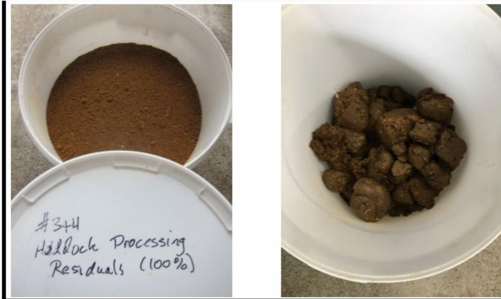
During a trial, 16 batches of haddock and whiting were run through the machine as whole fish, fish processing residuals and a combination of both. Of the 16 batches, all but 2 produced a dry powder like material (as shown above to the left); 2 batches of whiting processing residuals produced a more solid like product (as shown above to the right) due to its higher oil content.
