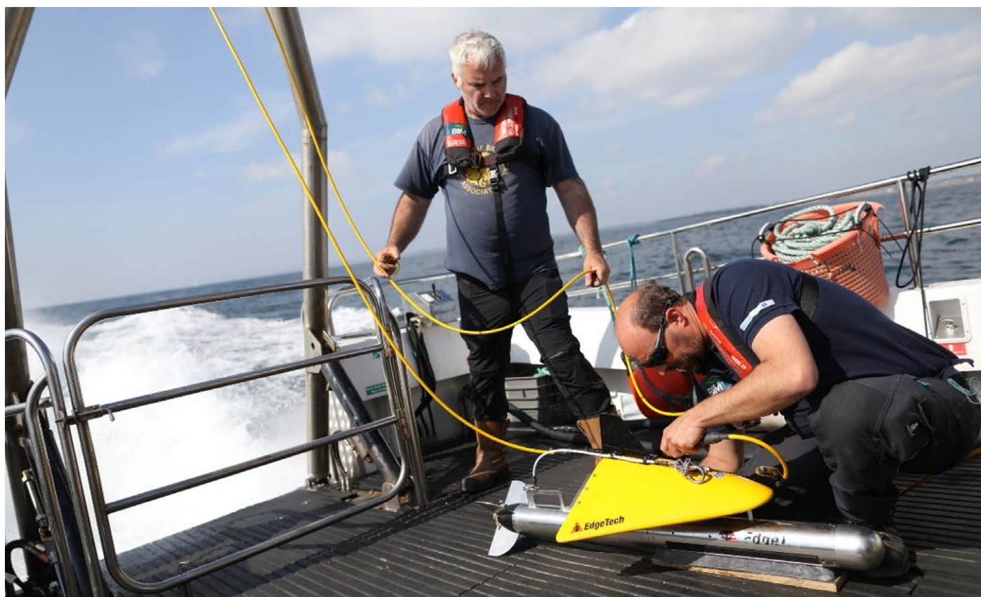
Figure 4. Towfish being prepared for deployment from the RV T. Burke II
