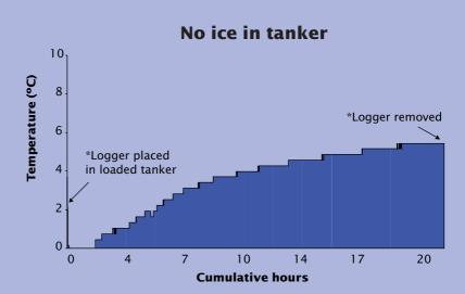
This graph illustrates how the temperature of fish in a loaded tanker rises rapidly, without the addition of slush ice.
