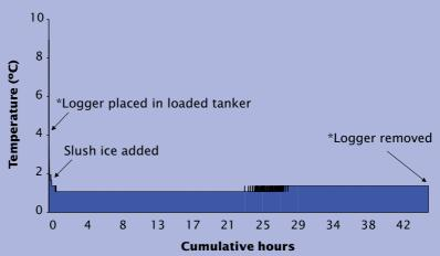
This graph illustrates how the addition of slush ice to a loaded tanker maintains good temperature management.
