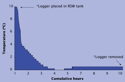
This graph illustrates good temperature management when fish are added to an RSW tank.
