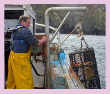
A derrick and snatch block is most commonly used to bring pots on board but some vessels also use a roller to bring the pot over the gunwale and land it onto a stainless steel table.
