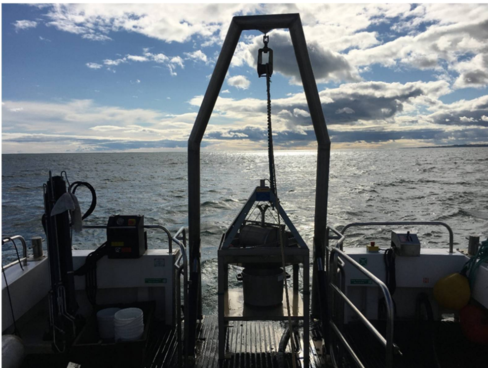
Day grab on the survey vessel deck
