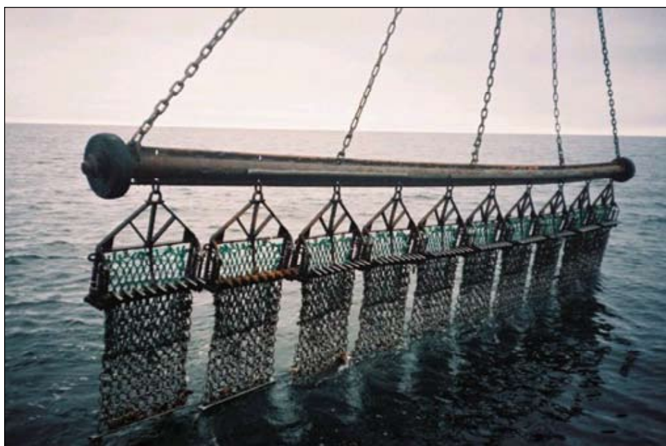
Figure 1. Commercial spring loaded scallop dredges suspended on a beam being deployed from a commercial fishing vessel.
