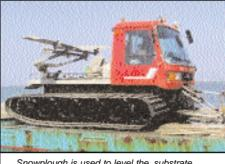
Snowplough is used to level the substrate
