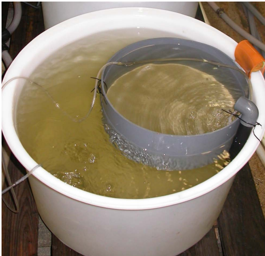
Figure 9. Settlement bin showing airlift pump and microalgal mixed ration
