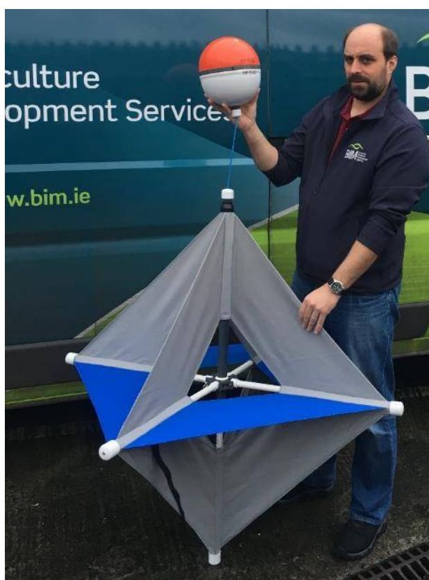
Figure 23: Detail of the Microstar GPS drifter
