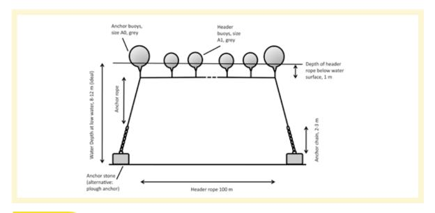
**Figure 3.2.**Diagram showing construction of a 100-m longline for seaweed cultivation (not to scale).
