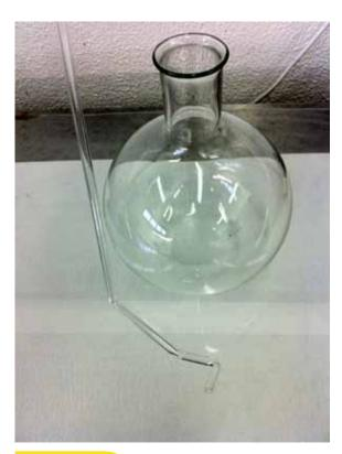
Figure 4.9. Modified glass tubing for scraping gametophytes from the sides of glass flasks.
