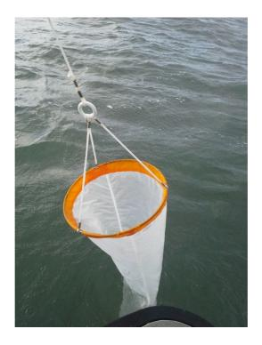
Fig. 4: Plankton net being deployed
