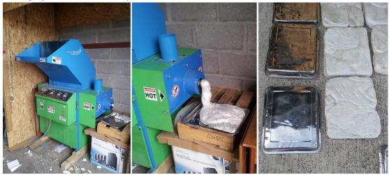
The EPS is fed manually into the machine; while it had been considered that a larger hopper could be designed to facilitate machine-driven feeding, PE advised that there needs to be attention paid to all material being processed and therefore manual intervention is necessary.
