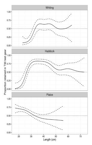
Figure 5. Predicted proportion of overall catch at length retained in the T90 test gear. Predictions are from generalized additive mixed models per species. Solid lines represent the predicted mean proportion and dashed lines the upper and lower 95% confidence intervals. Equal proportions are shown as dotted horizontal lines at 0.5.
