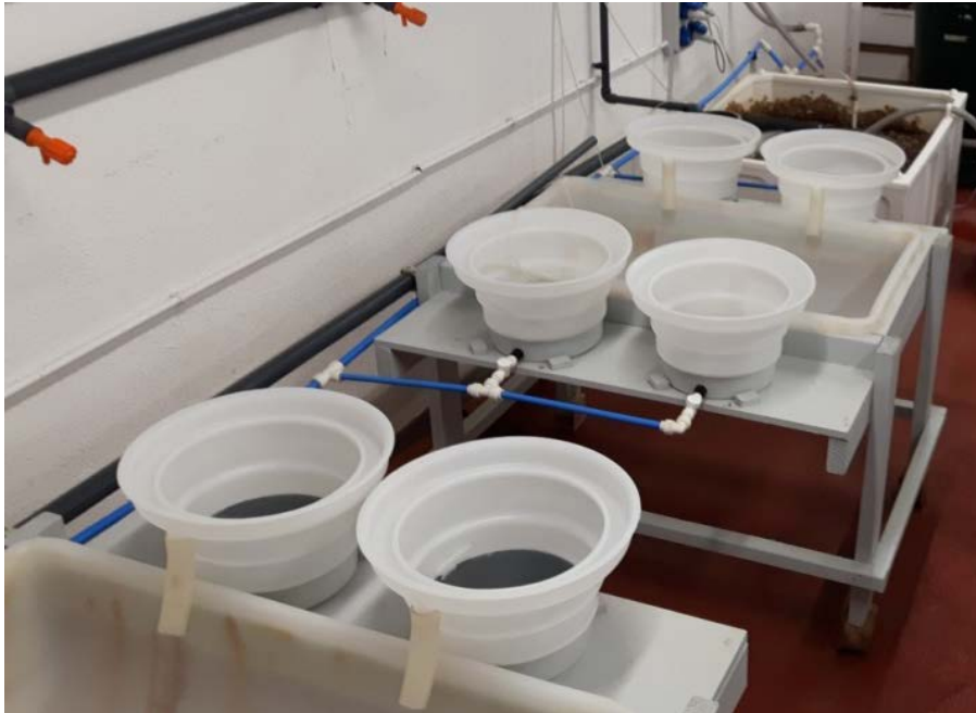
Figure 3. Lump sucker egg incubation system at Carna Research Station with holding tanks (150 L capacity) and sump (490 L capacity) filled with biomedica. System fitted to heater/chiller unit to control temperature (not pictured).
