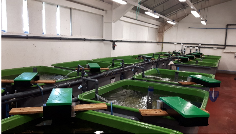
Figure 12. Belt feeders installed over larval/juvenile lump sucker tanks in Lab 2 at Carna Research Station.
